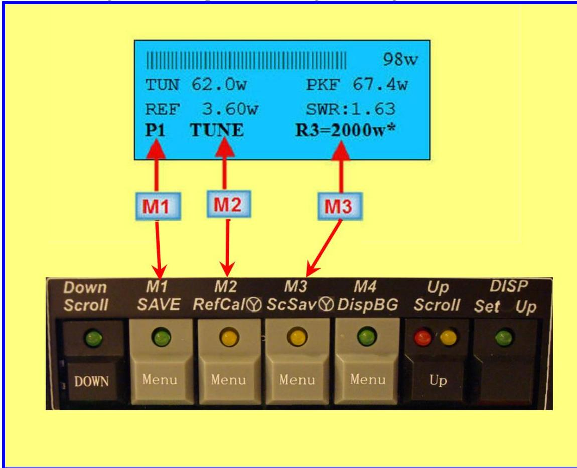
The example above shows the menu that controls the Analog Meter functions. Menu buttons M1 - M3 correspond to the three positional items on line 4 (*menu items are separated on line 4 of the LCD by one or more spaces*). The Panel Meter menu in this example has only three fields. Therefore, **M4** is not used with this menu.
