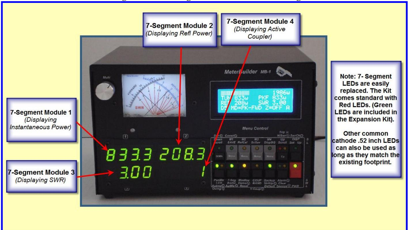
You can activate the Seven Segment Display menu using the **UP** or **DOWN** scroll buttons. Alternatively a short press of the 7-Segment shortcut button (described in detail below) will also bring up the Seven Segment menu immediately without the need to use the Up/Down scroll buttons. Use either method to bring up the 7-Segment menu on line 4 as shown below.
