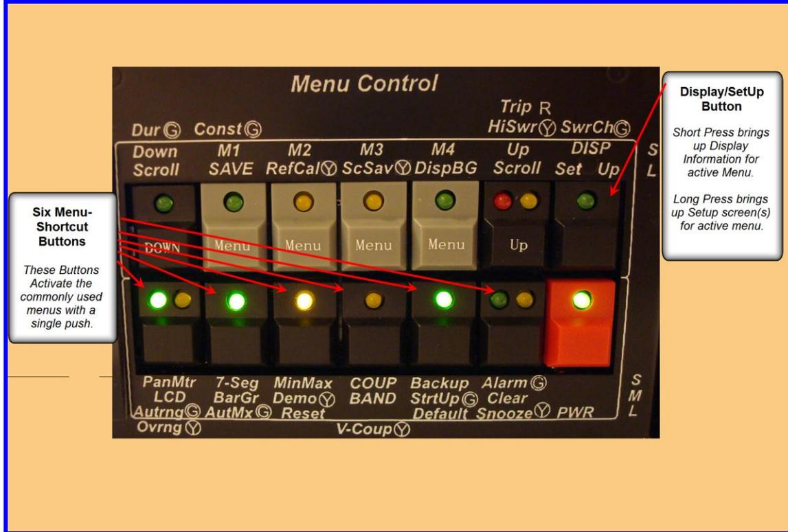
For example, the leftmost bottom button, **PanMtr/LCD/Autrng**, allows you to access *either* the Panel Meter Menu or LCD setup menu. A **short** press will bring up the first of the two menus (Panel Meter menu in this example). A **medium** press will bring up the second of the two menus (LCD setup menu in this example). The last function of this switch, **AutRng**, toggles the Panel Meter AutoRange function on and off when a **long** press is applied.
