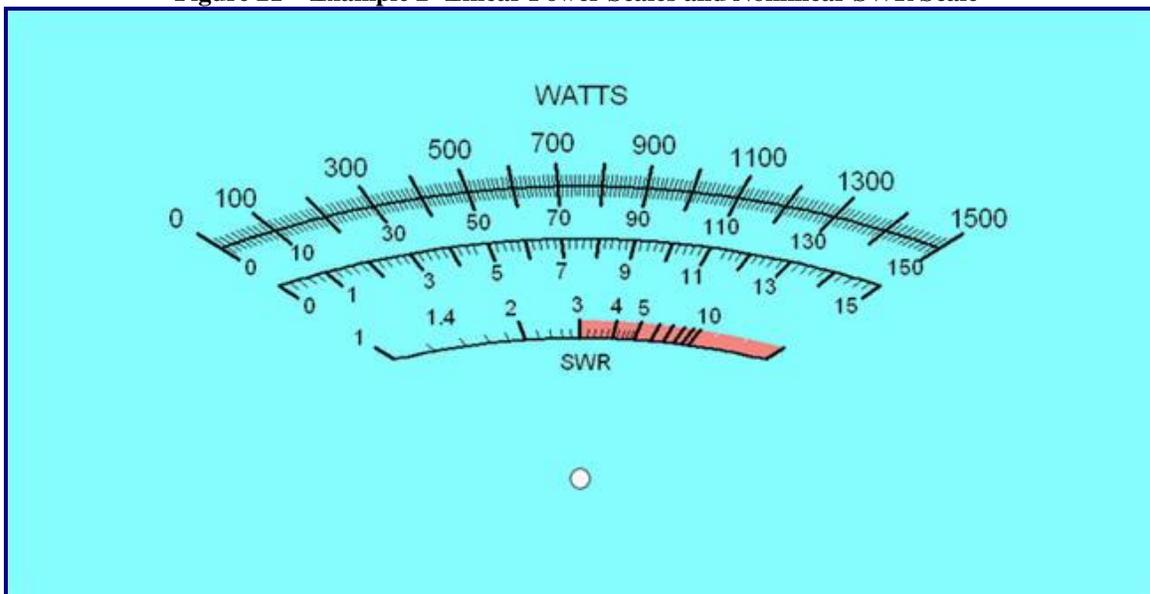
Figure 22 – Example 3 -Nonlinear Power Scale and Nonlinear SWR Scale
