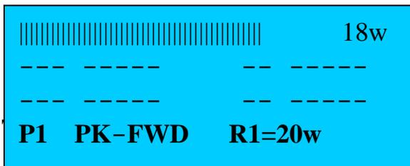
Bring up the Peak Hold Setup menu on line 4 using the **UP** or **DOWN** scroll buttons as shown below.
