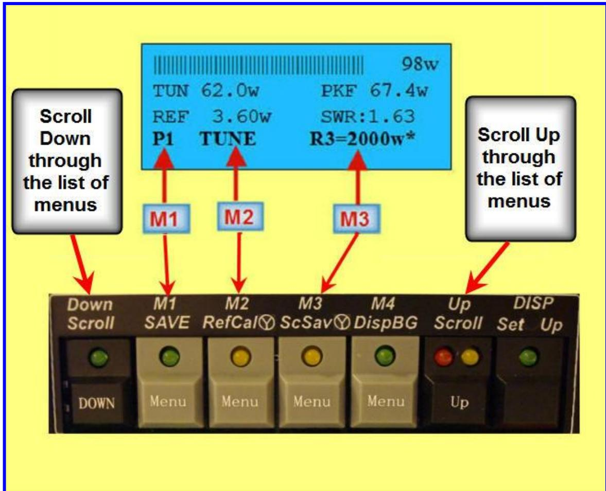
The example above shows the menu that controls the Analog Panel Meter functions. Menu buttons **M1** - **M3** correspond to the three positional items, as read from left to right, on line 4 of the LCD. (*Menu items are separated on line 4 of the LCD by one or more spaces.*)
