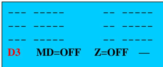
Once **D3** is selected, menu button **M2** is used to change the parameter to be displayed on the selected 7-segment module (which is displayed in the second field of this menu). Tap **M2** (second menu button) repeatedly until the second field of the menu is set to **MD=SWR** (mode = SWR). Again, if you overshoot, simply tap **M2** repeatedly until the **SWR** option appears again.
