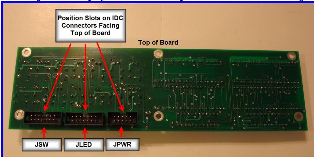
**Figure 12 - Controller Board – IDC Cable Designations**
