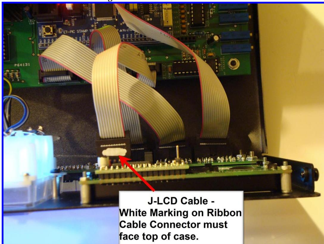
Three ribbon cables interconnect the Switch Display Board to the main controller board. These cables interconnect the **JSW**, **JLED**, and **JPWR** IDC connectors on the two boards. The **JMTRPOT** IDC connector connects to the ribbon cable that is wired to the analog crossneedle meter and 10 turn pot. The **JLCD** ICD connector connects to the 4x20 LCD.
