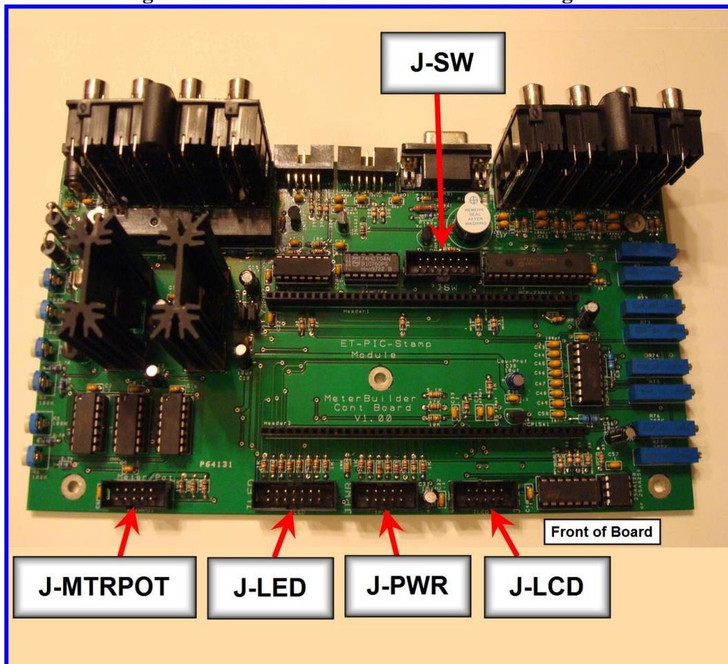
The microcontroller board plugs into the two 40 pin headers as shown in **Figure 13** below. The RS-232 signals are generated on the microcontroller daughter board, and connect to the main controller board with the two jumpers as show below.
